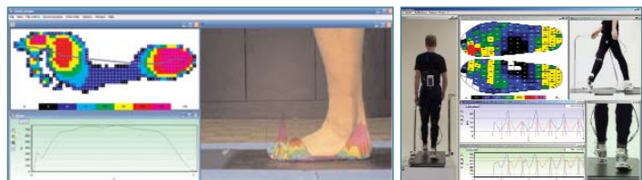
video with overlaid 3D pressure distribution display
